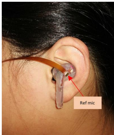
Figure 1 TWS mockup on ear and location of reference microphone
